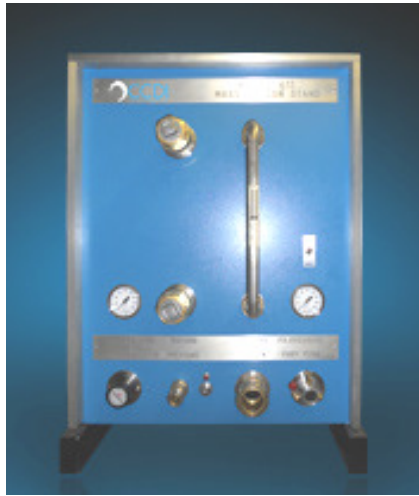
Model 611 NIST EFA Machine Test Stand Dimensions: 33" H x 24" W x 22" D 838mm H x 610mm W x 559mm D
